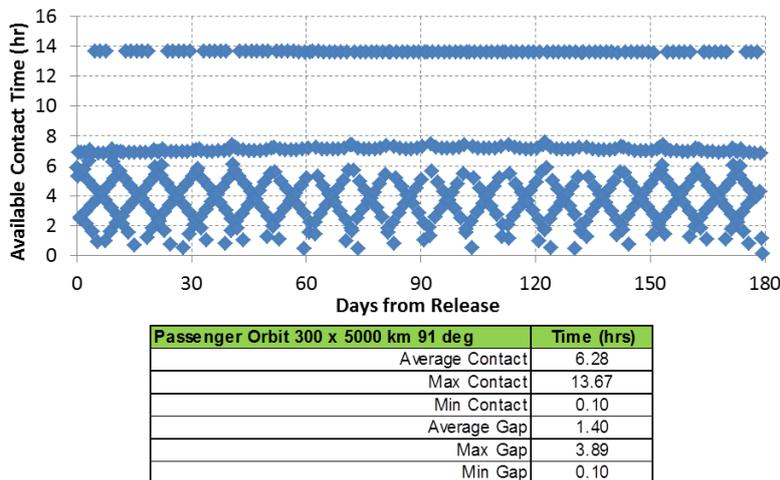
**Figure 4-2: Example of total contact time available between a passenger in a 300 x 5000 km lunar orbit and the Mothership.**
